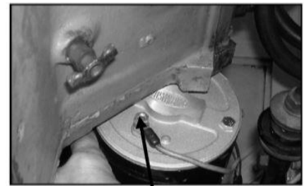
Battery Output Terminal
